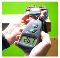
Grow Bright digital lux meter HTG Supply ACC-GBLM100 http://www.htgsupply.com/Product-GrowBright-Digital-Light-Meter
