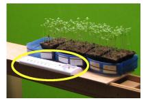
Placing the humidity meters side by side revealed that they tended to report slightly different humidities at the same time and place. I compared the humidity readings side by side on 3 days, and estimated that the average difference was only 1% (with a standard deviation of +/-2%). I normalized the reported humidities accordingly.
