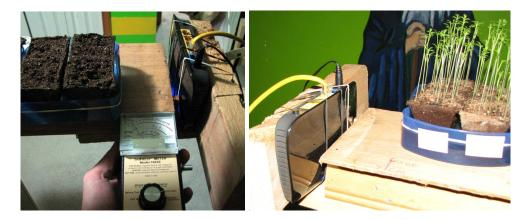
I tested if garden cress was affected by a WIFI signal strength above  $\frac{0.1 \, uW}{cm^2}$  <sup>9</sup>. This is easier said than done.  $\frac{0.1\,uW}{cm^2}$  is less than my electro magnetic field (EMF) meter can detect, which I worked around by holding my meter closer to the WIFI router, and using the inverse square law to extrapolate how low the signal strength should be at greater distances<sup>10</sup>.
